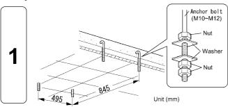
Embed off-the-shelf anchor bolts (M10 $\sim$ M12) at the ceiling suspension fixture mounting positions beforehand, referring to the outside dimension drawing and the example of installation as shown above.
