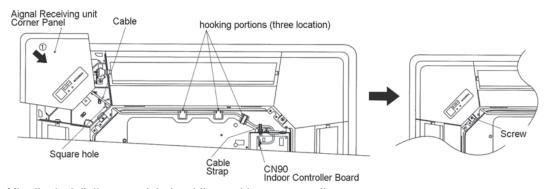
$\bullet \mbox{After the installation completed, set the cont,box cover as they were.}$
