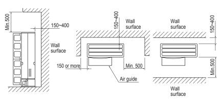
(2)Multiple unit installation : Installation of multiple units in series must be no more than 5 units.
